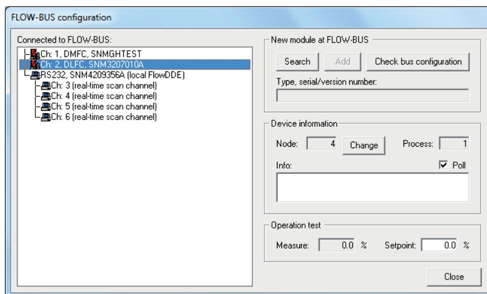
On the left hand side, all instruments connected to the FLOW-BUS are shown, ordered by their assigned channel. In this example, two digital controllers (channel 1 and 2) and one RS232/FLOW-BUS interface with 4 real-time channels (channel 3 to 6) are connected.
